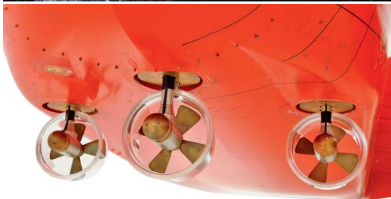
Pieter Schelte model is equipped with 12 independently operating thrusters
